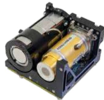
performance, and long life with high MTBF, delivering high quality images for a wide range of tactical applications. Based on SCD's 640x512 10  $\mu$ m FPA with mature XBn HOT (High Operating Temperature) technology, the Sparrow solution operates at 150K, enables extremely high quality images, best in class SWaP, and low cost. This video core enables implementation of
